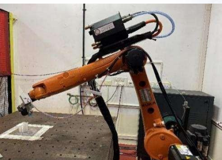
Standard Robotic cell intergrated with complete MIG welding unit from KUKA robot
