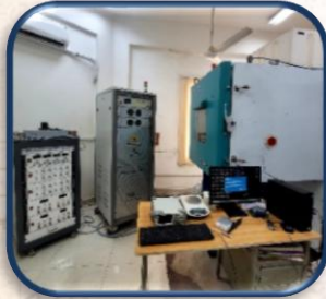
Vibration Test Rig with environmental Chamber
